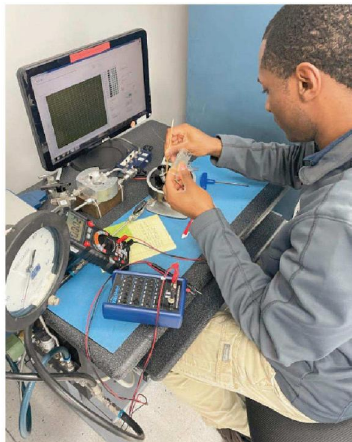
In-House Sensor Assembly And Calibration For Smart Valves
